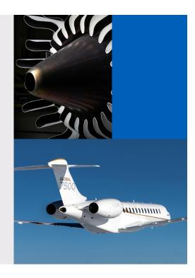
Setting new standards for ultra-long-range business jet reliability and efficiency Sporting a thrust just under 19,000 pounds, GE's Passport engine powers Bombardier's latest and most elite ultra-long-range business jet, the Global 7500. Designed and built for range and comfort, Passport incorporates a blend of technology created and honed by GE over decades of experience and success in commercial and military engine design.
